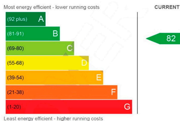
Figure 17. New EPC rating post-retrofit solution.
