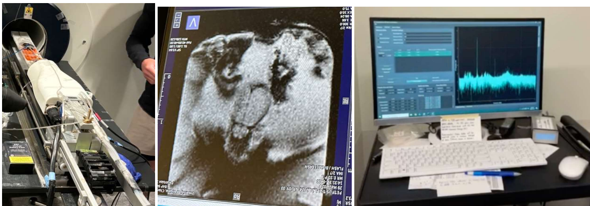
Figure 10. Left. Mouse placed on the RK-300 FUS device before being introduced into the MRI and PET scanners. Center, MR image of the mouse brain before sonification. Right spikes observed when the FUS were being applied.
