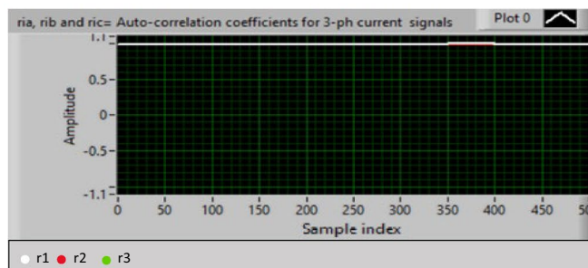
(c) The auto-correlation coefficients ( r_{ia} , r_{ib} and r_{ic} ) for three phase secondary current signals
