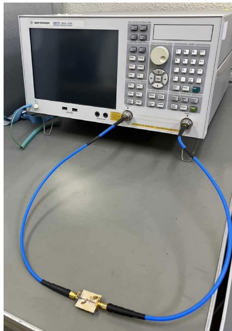
Fig. 14 The measurement setup of the fabricated CRLH-TL BPF
