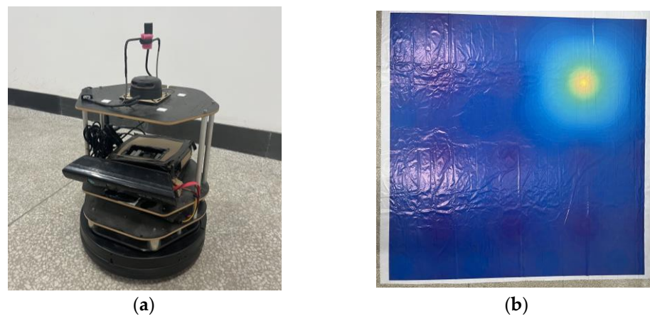
Figure 11. TurtleBot 2 and the map used in the experiment: (a) TurtleBot 2; (b) the map printed with a contour plot of the Ackley function with the coefficients a = -36 , b = 2.2 , and k = \pi . The global maximum is indicated with a color of bright yellow.
