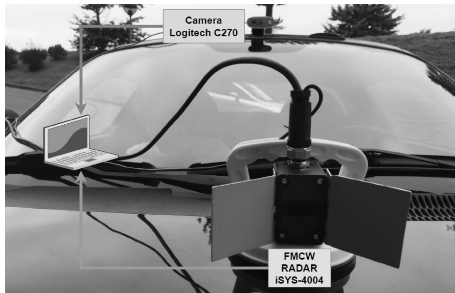
Figure 5. Mounting of the radar on the vehicle.
