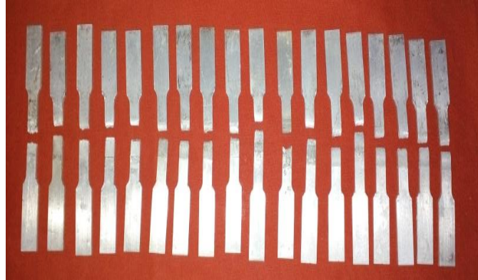
Figure 1 Tensile specimen after testing
