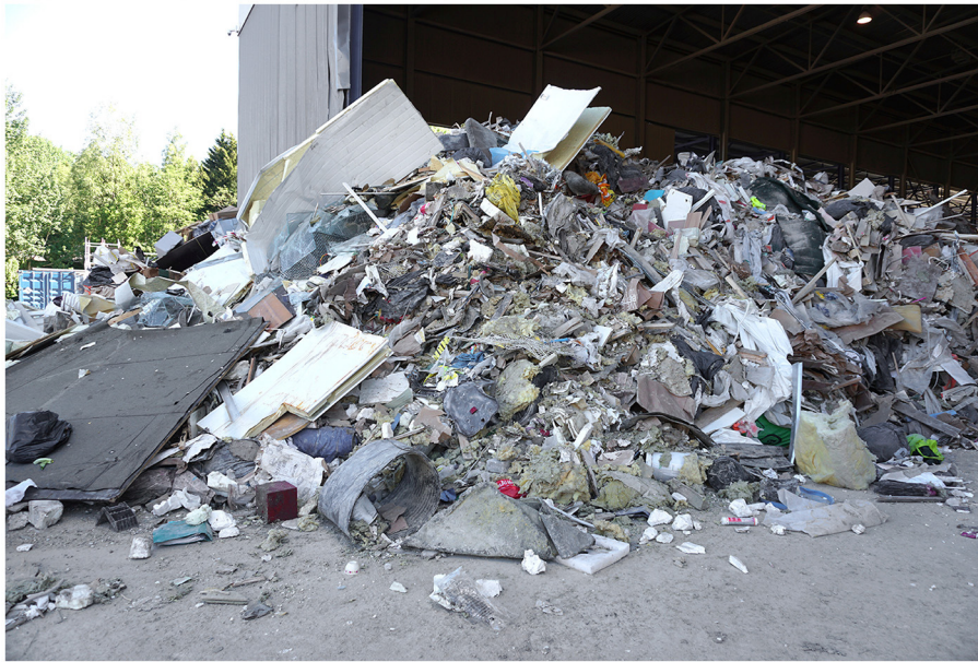
FIGURE 1 A pile of mixed demolition waste containing plasterboard.
